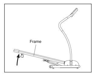
2. Raise the frame slightly and pull the latch knob to the right. Pivot the frame upward and release the latch knob. Raise the frame until the latch knob locks into the storage position. Make sure that the latch knob is locked in the storage position.
